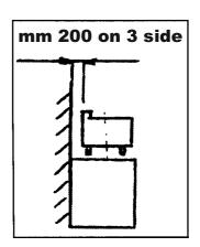
Adequate ventilation is essential for safe operation of a gas appliance. A supply of fresh air is necessary for the correct combustion of the gas and there must be a means of exhausting the heat and the products of combustion from the kitchen. It is recommended that the appliance be sited below a ventilating hood, one preferably connected to an extractor system incorporating a grease filter.
